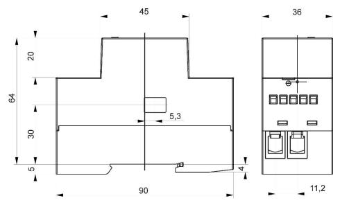
Figure 2: Dimensional drawing and rear connection terminals position
