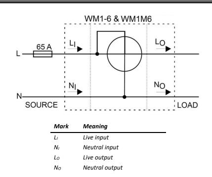
**Figure 3:** Electrical diagram 230 V<sub>AC</sub>
