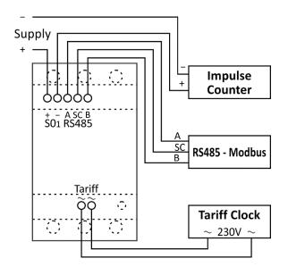
**Figure 6**: Connection diagram of SO output, impulse counter, RS485 - Modbus and tariff clock
