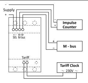
**Figure 7**: Connection diagram of SO output, impulse counter, M - bus and tariff clock
