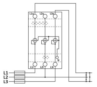
**Figure 3**: Three-phase 3-wire 2 system connection diagram (2W3)
