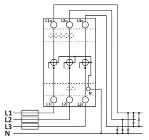
Figure 1: Three-phase 4-wire connection diagram (3W4)
