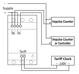
**Figure 5**: Connection diagram of SO output, impulse counter, impulse counter or controller and tariff clock
