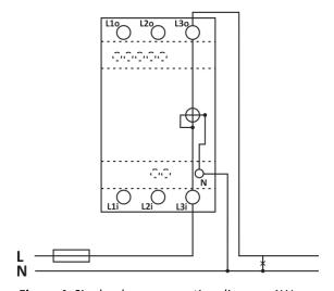
Figure 4: Single-phase connection diagram 1W
