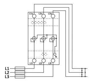
**Figure 2**: Three-phase 3-wire 3 system connection diagram (3W3)
