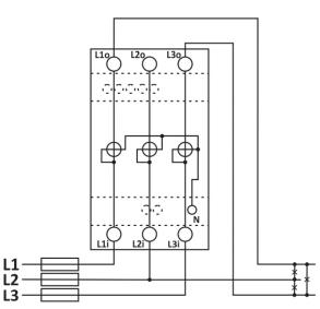
Figure 4: Three-phase 3wire 3 system connection diagram (3W3)
