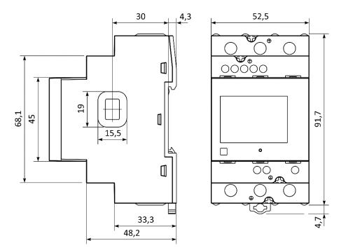
Figure 2: Dimensional drawing and rear connection terminals position
