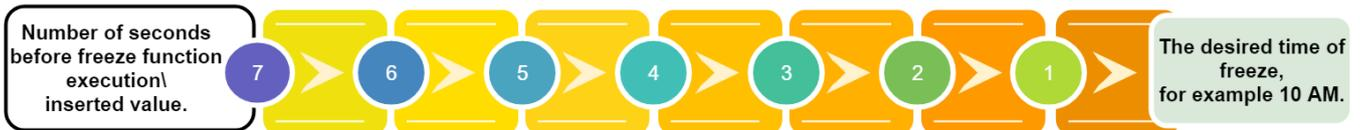
All instruments that received one of the commands will freeze at the same time. This is the advantage of the described register, so it is recommended to use it.
