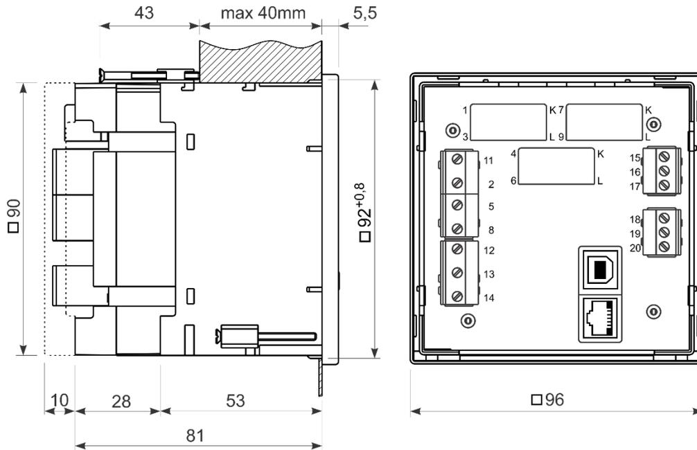
Dimensions for iMC750 (terminal connection assignment):
