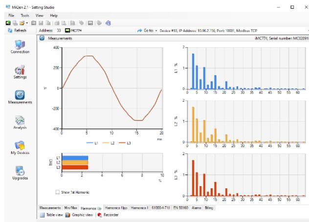
Figure 3: The sample of online harmonic measurements in graphical form
