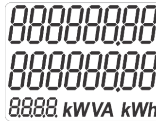
Figure 6: LCD segment test
