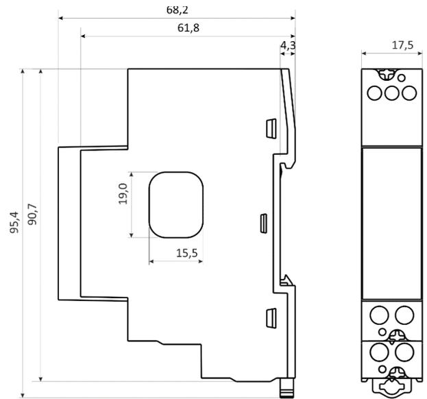
Figure 3: Dimensional drawing of IE14
