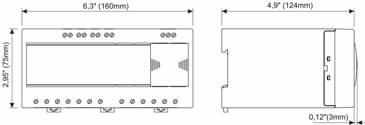
Dimensions for iMT550/560 (ring type terminal block):
