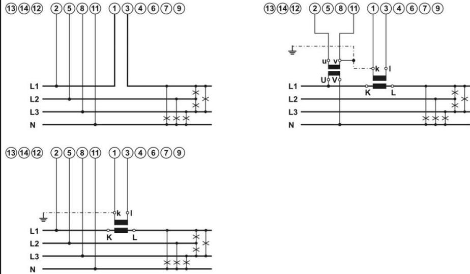
Three-phase four wire connection with unbalanced load
