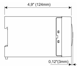
Dimensions for iUMT540 (ring type terminal block):
