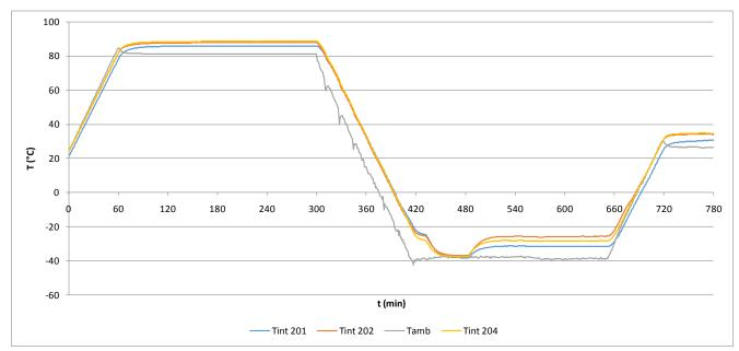
The meter 19200201 connected single phase after reconnection at -40 °C
