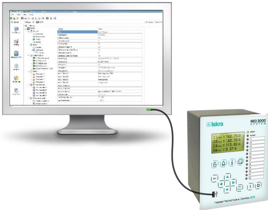
Figure 4.41 Connection between FPC device front port and PC via USB male - A to male - A.
