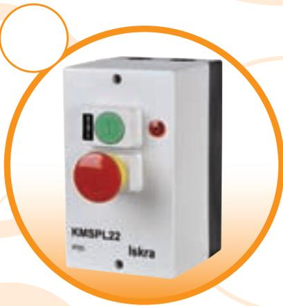
They are mainly used for start-up and switch-off of electric motors up to 11 kW power. MS25 motor protection switch with undervoltage release and a corresponding contactor are built in the enclosure of degree of protection IP55.
