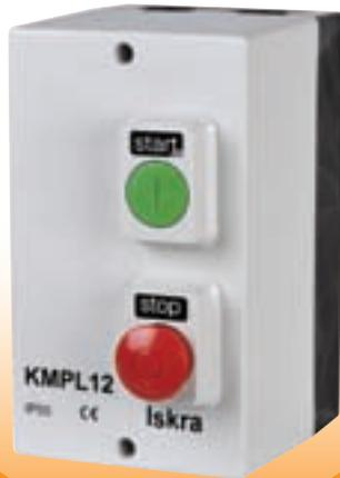
They are mainly used for start-up, overload protection and switch-off of electric motors and also for other loads. A contactor and a corresponding bimetal relay are built in the enclosure of degree of protection IP55. They are switched on with the ON pushbutton and switched off with the OFF pushbutton. The mushroom pushbutton functions as an emergency stop pushbutton.
