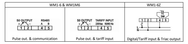
RS485 serial communication with the MODBUS protocol, which enables data transmission and thus connection of the measuring places into the network for the control and management with energy. They can also be equipped with tariff input (option). Both supported only on WM1-6 and WM1M6.
