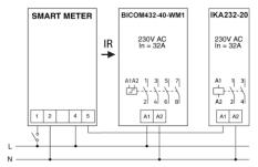
Picture above indicates connection of two external relays to WM1-6Z. BICOM432-40-WM1 connected via optical (IR) communication port and IKA232-20 connected via Triac output.
