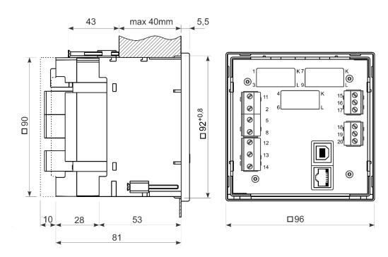
Dimensions for MC 740 (terminal connection assignment):
